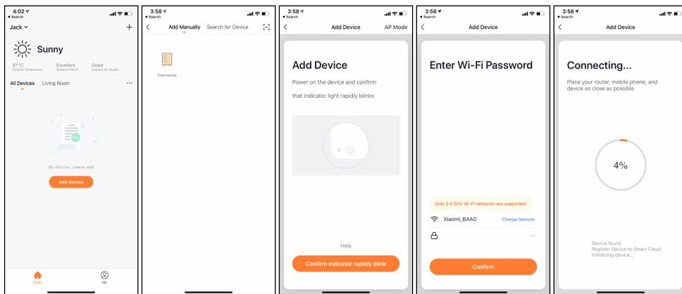
**Step1:** Turn on the power of the heater by pressing the Power Switch. The WIFI signal will start to flash rapidly. Open the APP on your smartphone and add your device. Choose “Add Device”, then “Add Manually”, and then choose “Thermostat” to add the device.
