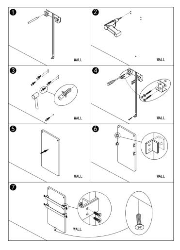
Step 1. Use the mounting bracket to mark the position of the hole on the wall.
